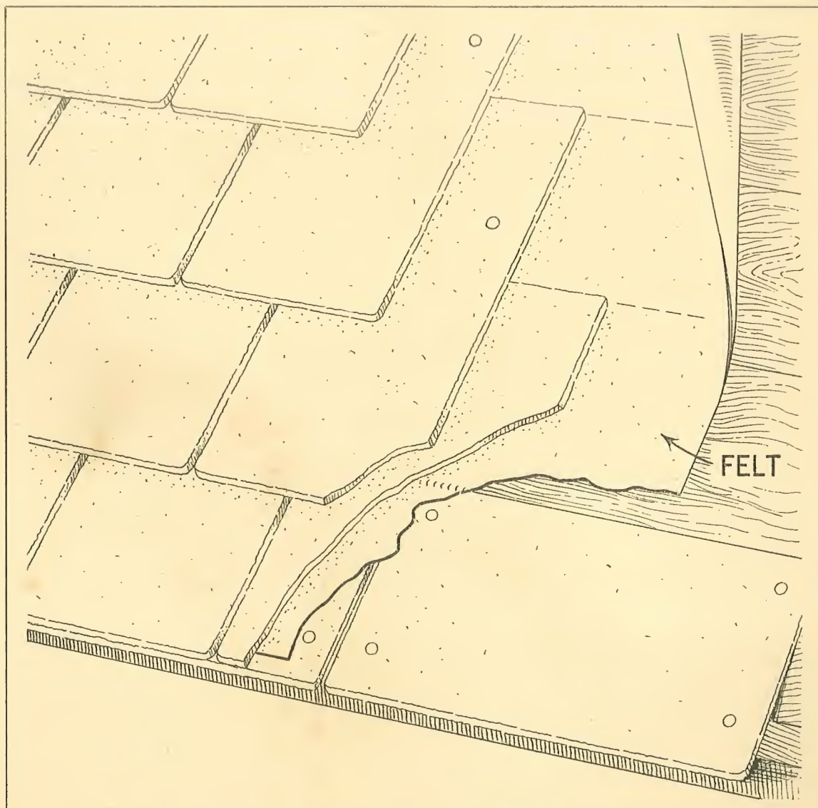
Figure 13—Showing Method of laying American Shingles with even butts
